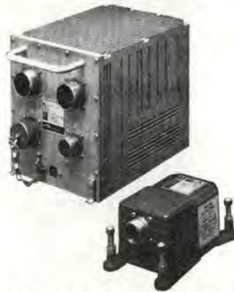
F-16C/D and F-15E aircraft will soon have crash survivable FDRs. The F-16 Signal Acquisition Unit (pictured above — top) records aircraft information and transmits this information to the F-16 Crash Survivable Memory Unit (pictured above — below).
